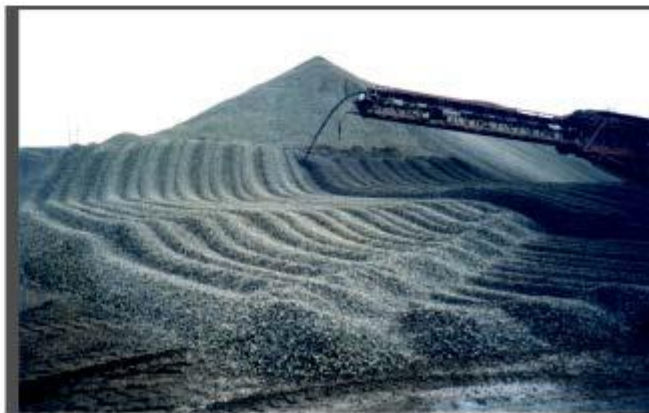
CREATING WINDROWS WITH A TELESCOPING CONVEYOR F23
