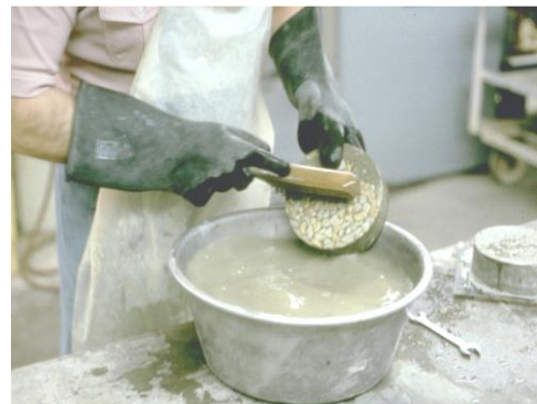
Preparing a sample for the circular track
