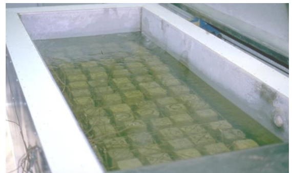
Test beams are run through 350 cycles
