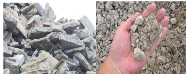
Uncrushed & Crushed Recycled Concrete
