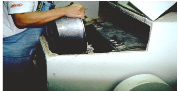
6) Material is placed in the LA Abrasion machine
